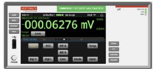
The DMM7512 virtual front panel displays a conventional DMM front panel.
